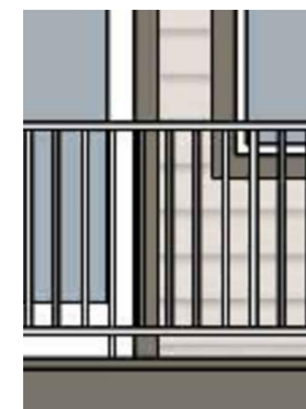
METAL GUARDRAIL PAINTED SW 7042 SHOJI WHITE
