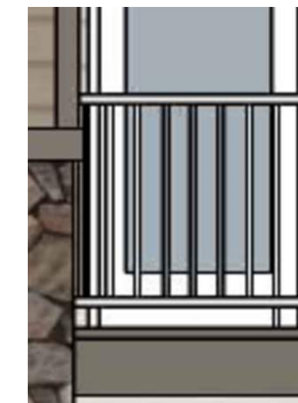
METAL GUARDRAIL PAINTED SW 7042 SHOJI WHITE
